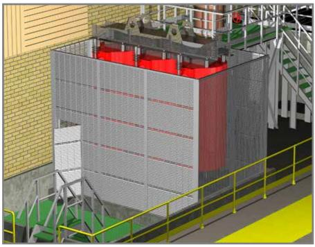
Protective Screen system incorporating safety door and featuring both louvred panels for security and safety to front and Open Grid for easy inspection to side.
