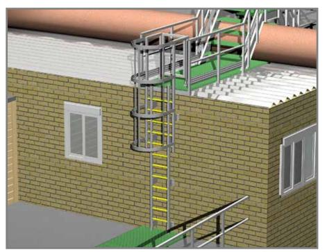
Illustration to show how access to a roof can be gained safely using a ladder system incorporating a safety cage and walk through
