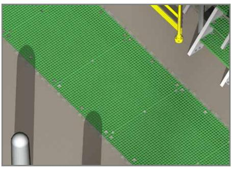
Moulded FRP Grating green structural walkway allowing safe passage above trench carrying surfaces that require ventilation
