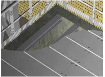
Cut away revealing I Beam FRP Chamber Cover supports
