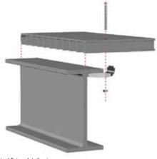
Typical fixing detail using dome head washer
